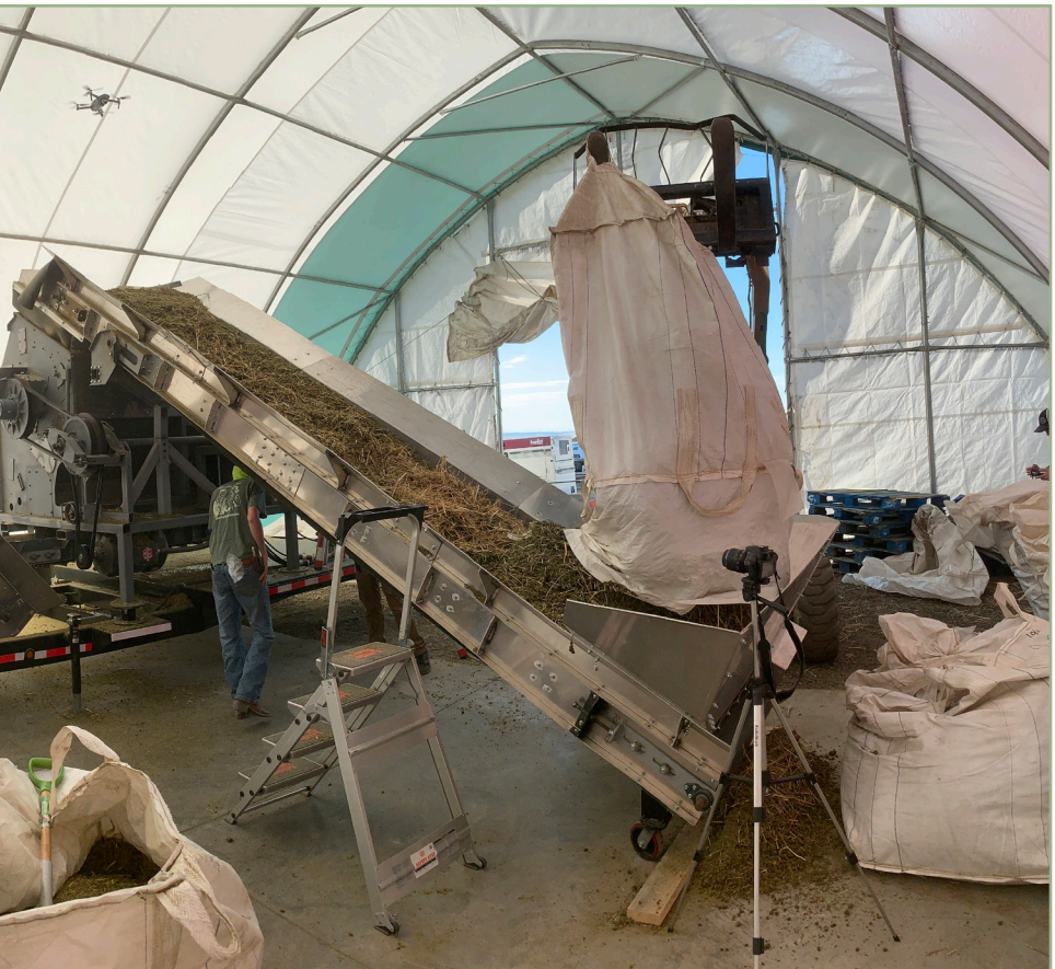
A Bish hemp separation system.
